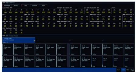
• For consoles with an external monitor connected, the Faders window can be viewed on the bottom half of the Faders desktop.
