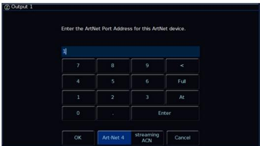
You can also remotely configure the individual DMX Output ports of the gateway using the "Outputs" fields. This allows you to choose which Art-Net universe that physical port will output. For example, you may configure all the ports to output Art-Net universe 1.
