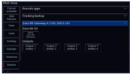
In this image, Zero 88 Gateway 4 can be seen by ZerOS. This is how most Ethernet to DMX gateways (sometimes referred to as "nodes") will be displayed in Devices.
