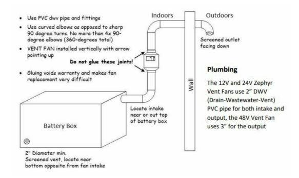
For the inquisitive, please note that the 48 volt Vents Fans are built with two 24 volt fans wired in series.
