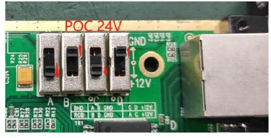
• POC function OFF: Have the 4-pin DIP switch set to the middle position.
