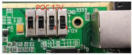
• Set POC to 24V: Have the DIP switch A & C down, and the B & D to up position.
