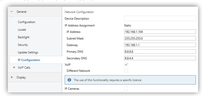
Irrespective of the video intercom to be used, the following configuration is required in ETS for the indoor unit. First, the IP configuration of the device must be set by configuring a static IP within the network range and enabling VoIP functionality from the "IP Configuration" tab.
