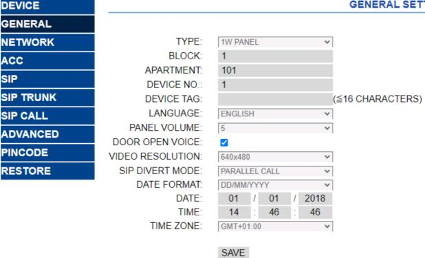
In case of calling several indoor units simultaneously, you can select the PARALLEL SIP FORWARD MODE to call them at the same time or SEQUENTIAL to call one after the other if it does not answer within 30 seconds.
