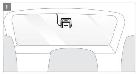
2. Peel the protection film of the sticky pad and camera lens. Fix the rear camera on the selected location and adjust the lens.
