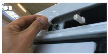
4. Route the main cable from the infotainer in the vehicle cockpit/dashboard to the brake light opening in the upper rear section of the vehicle. Fore power and RCA video signal, the ZENEC infotainer offers a direct system "connector block E" which offers switched 300mA power out's (see installation guide of ZENEC head unit).
