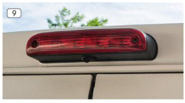
9. Alignment of the camera ball at the bottom side of the camera main body if necessary, using the supplied U-shaped tool
