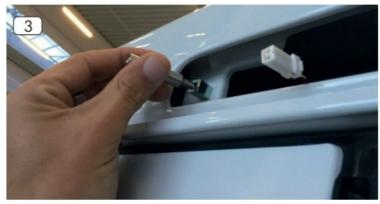
5. Insert the brake light assembly into the main housing. Next, plug in the white power supply system connector into the socket on the brake light reflector housing backside. Connect the mini-4PIN connector of the cam sensor end to its counterpart of the extension cable.
