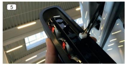
6. Align the cam housing / reflector assembly over the mounting location. Fix the assembly with the original Philips head screws.
