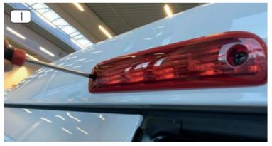
2. Pull the brake light reflector unit out of its mounting slot. Disconnect the white power supply system connector plug of the vehicle.
