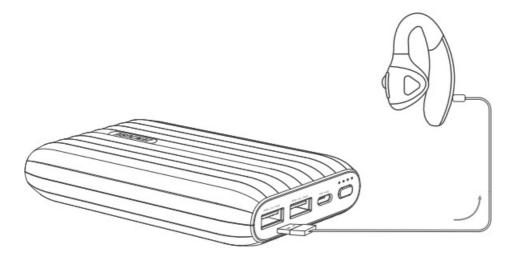
Double press power button, X5 will enter X-Charge mode and LED indicator will show as follow. Connect your low-current devices to the USB-A output ports of X5 with a charge/sync cable and they will be continuously charged. Double press power button again to quit X-Charge mode.
