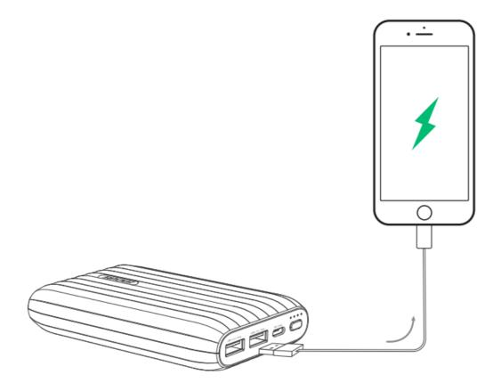
Connect your device to the USB-A output port of X5 with a charge/sync cable. As the device is being charged, the LED indicator display the power level.
