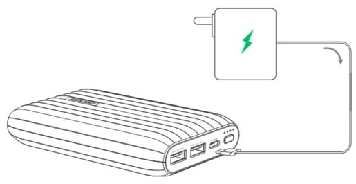
Connect the power adapter to the USB-C PD port of your X5 with a USB-C charge/sync cable. During charging, the LED indicator will flash and display the charging power level.
