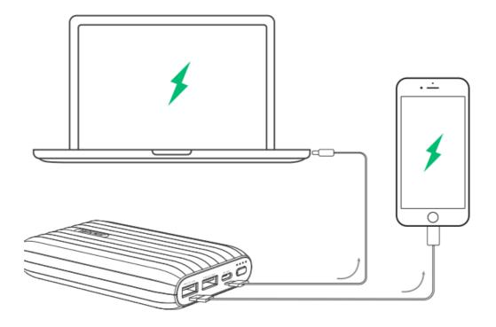
Connect the USB-C Hub port of X5 to USB-C port of your laptop with USB-C to C cable. Double click the power button, and X5 will enter USB hub mode, you can sync and manage your files with 2 USB-A ports. Double click
