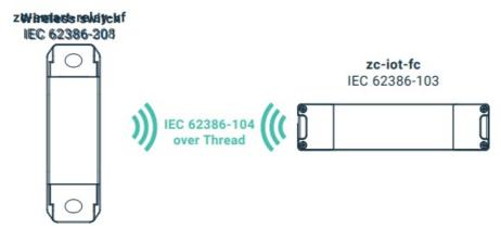
2. 104 + 101 Bridge mode is enabled after the device has been added to a 104 controller and a 101 power supply has been connected to the DALI terminals.
