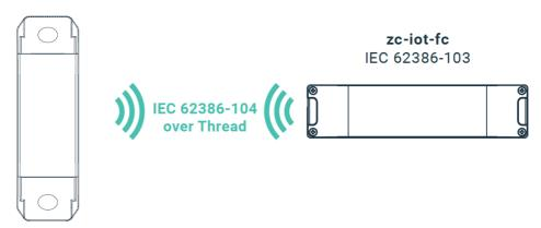
2. 104 + 101 Bridge mode is enabled after the device has been added to a 104 controller and a 101 power supply has been connected to the DALI terminals.
