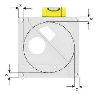
• Fix the bottom cover in place in the four fixing points on the façade.
