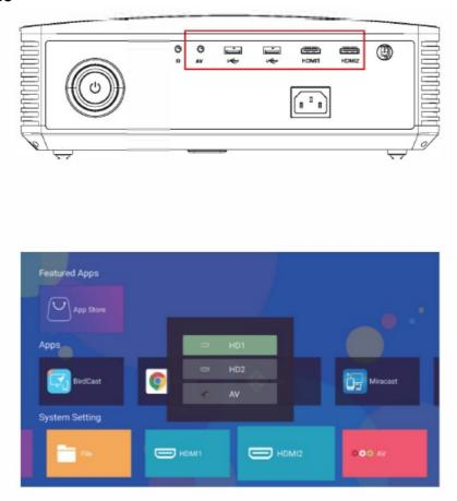
Once the HDMI / AV is connected to the projector, you will need to select the specific signal source as the input. After connection the content played on the source will be streamed on the projector.
