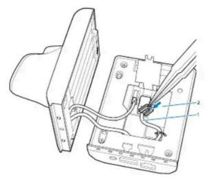
9. Reapply the sticker, ensuring it holds the new cable jack and plastic bezel in place.
