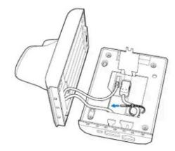
8. Position the plastic bezel between the cable (1) and the PCB (2).
