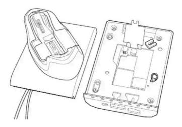
7. Connect the new USB cable to the connector on the base. Secure the cable to the base with a new cable tie and position it under the middle frame. Connect the power cable to the connector on the base.
