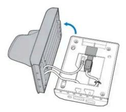
3. Using scissors, cut the cable tie and release the cable
