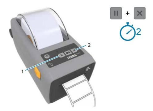
Press and hold the Pause (1) and Cancel (2) buttons for two seconds to line up the labels.
