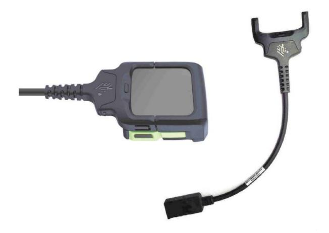
CBL-WS5X-USB1-01: WS50 charge cable. Provides charging and communications. Snaps on to bottom of WS50 device. Cable length 6 inches / 15cm. USB-C female port enables client-host connectivity. Requires separate purchase of USB-C cable and AC power adapter.
