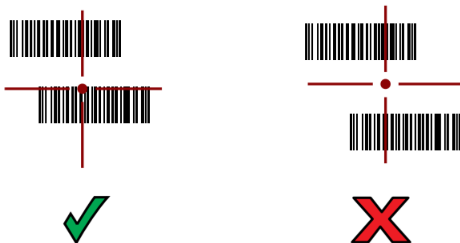
Figure 22 RS6000 Pick List Mode with Multiple Barcodes in Aiming Pattern
