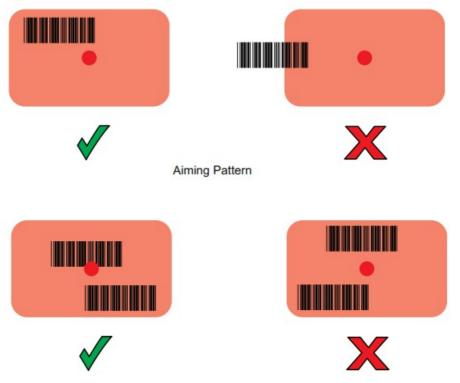
Pick List Mode with Multiple Barcodes in Aiming Pattern
