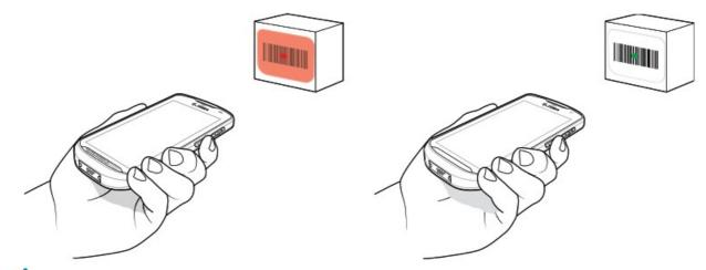
**NOTE:** When the device is in Picklist mode, the imager does not decode the barcode until the crosshair or aiming dot touches the barcode.
