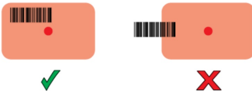
Figure 4 Pick List Mode with Multiple Barcodes in Aiming Pattern
