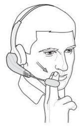
Place the microphone two finger's width away from the corner of your mouth, so it is slightly to one side.
