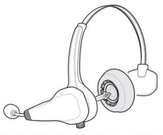
Firmly grip and pull the ear pad and inner casing.
