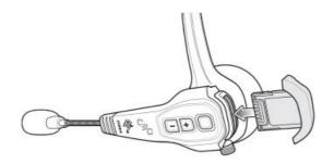
Insert the battery with the contacts facing outward.
