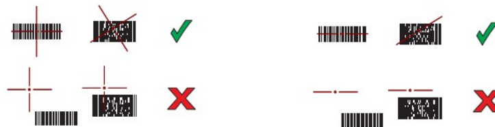
Figure 29 Pick List Mode with Multiple Barcodes in Aiming Pattern: Standard and Extended Range
