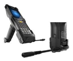
CBL-MC93-USBCHG-01: USB cable, provides fast-charge when a MC93 PP+ battery and a wall adapter is used, it also allows USB communication to the device when connected to a PC. Requires: CBL-TC2X-USBC-01 and Power supply PWR-WUA5V12W0US
