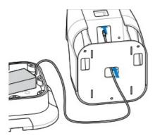
**5.** Pull the DC power cable up through the vertical stand body and then push it through the slot in the front of the VESA mounting plate.
