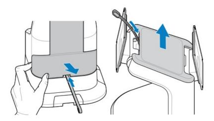
d) Use the removal tool to remove the two covers from the back of the KC50. Set them aside.
