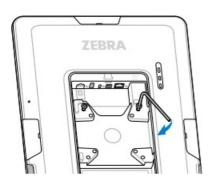
3. Connect the USB-C cable to the USB-C display port.
