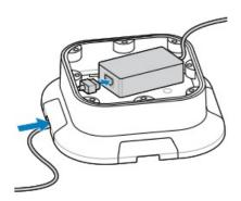
**NOTE:** If your setup requires any additional cabling (such as an Ethernet or second USB-C cable), include them in steps 3-11 and connect them to the KC50 once it is secured to the stand)
