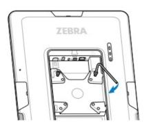
**10.** Hang the KC50 on the VESA mounting plate by sliding the two screws into the VESA screw slots.
