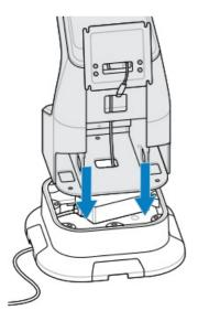
9. Loosely screw the two top screws into the 100×100 frame on the back of the KC50.
