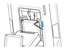
12. Connect the AC power cable to the DC power port on the back of the KC50.
