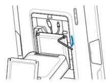
7. Secure the bottom of the TD50 to the VESA plate by attaching the two remaining screws.
