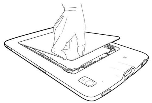
3. Insert the tabbed end of the expansion back into the battery well. Ensure that the tabs on the expansion back are aligned with the slots in the battery well.
