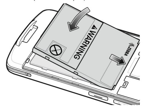
**NOTE:** When installing an extended battery, make sure to use the extended battery cover (KT-EC5X-EXBTYD1-01).
