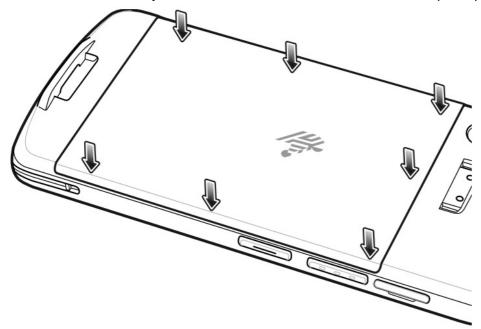
Follow the same steps to remove or install the extended battery and extended battery cover.
