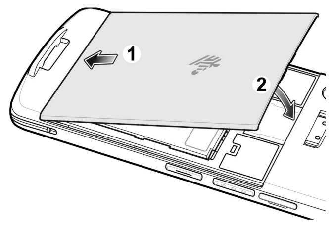
6. Press the sides of battery cover down until the notches on the sides snap into place.
