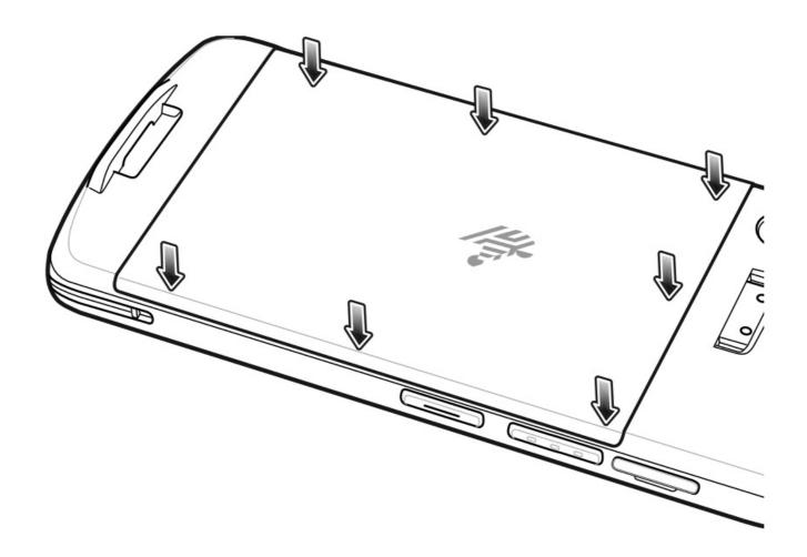
Follow the same steps to remove or install the extended battery and extended battery cover.
