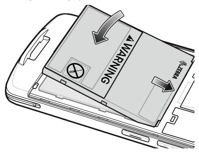
**NOTE:** When installing an extended battery, make sure to use the extended battery cover (KT-EC5X-EXBTYD1-01).
