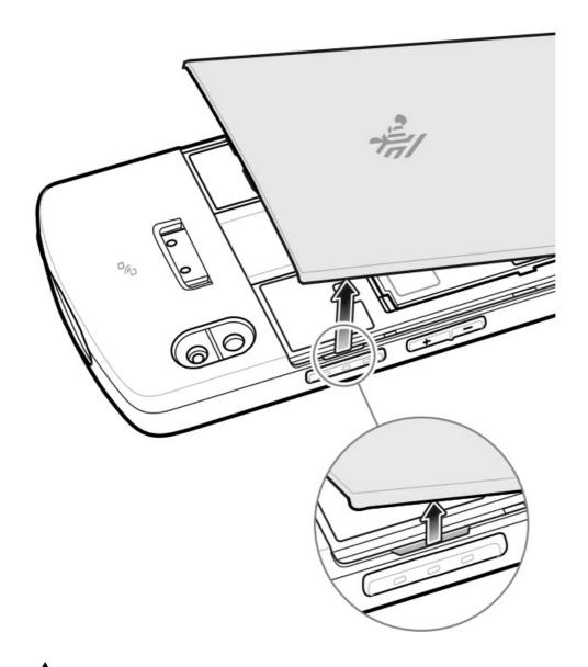
**CAUTION:** Do not use any tool for battery removal. A battery puncture may cause a hazardous condition and a potential risk of injury.
