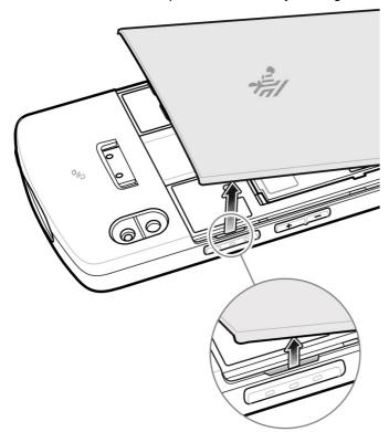
**CAUTION:** Do not use any tool for battery removal. A battery puncture may cause a hazardous condition and a potential risk of injury.
