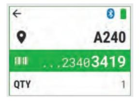
This application enables warehouses/manufacturers to easily increase the granularity of their inventory data. A worker scans an item, then uses the keypad and color display to add the quantity and location. For example, when workers put away new inventory, they can specify the aisle and shelf.
