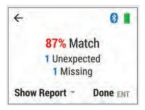
This application streamlines and error-proofs receiving tasks. A worker scans the shipping label on the outer container, then scans each individual item inside. The display confirms if the barcodes listed on the outside of the container match the barcodes on items inside.
