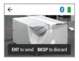
This application helps ensure high quality images when documenting damage on incoming shipments or equipment on the manufacturing line. After workers capture an image, they can preview it on the color display — then either choose to send the image to the host or discard it and take another.
