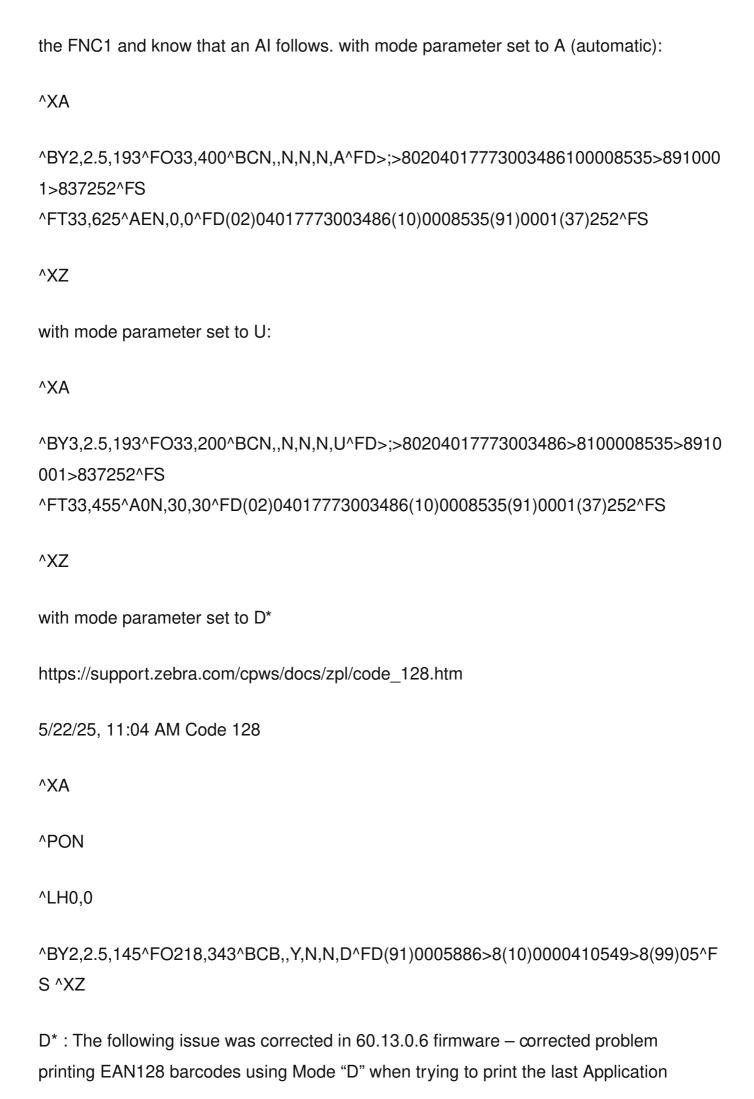
Identifier with an odd number of characters. The fix – Added in the capability for Mode D to accept odd numbers of data characters rather than trying to force an even number.
