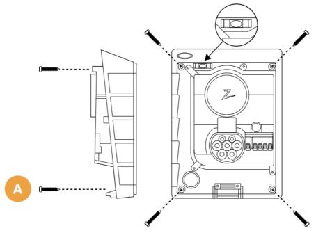
3. Place the power cable Choose between three entry options (top, back, and bottom) . Punch out the knockout tab to install from 1 or 2.
