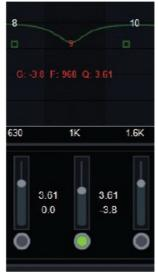
• You can click into the Gain or Q value box of any band and adjust using the up/down arrow keys.
