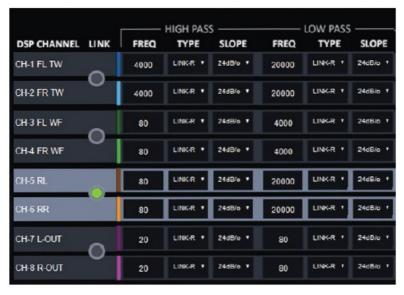
You can select a channel to tune by clicking on the desired speaker in the car diagram/Delay section or by clicking on its box in the DSP Channel column. You can pick channels on at a time or you can pick them by pair. Double-clicking the dot between a pair of channels links that pair. Similarly, if one channel is already chosen and active, then clicking on the dot will pair them.
