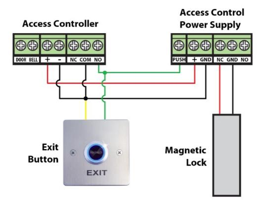
Exit buttons are used in access control systems to provide a momentary contact signal to the access controller to open a magnetic lock. This example shows a "Fail-safe" scenario. When the exit button is activated the access control power supply then releases power from the lock, and if power is lost then the lock also releases. Wire in NO or NC depending on the access controller used and also on the required state of the lock during a "Failsafe" or "Fail-secure" scenario.
