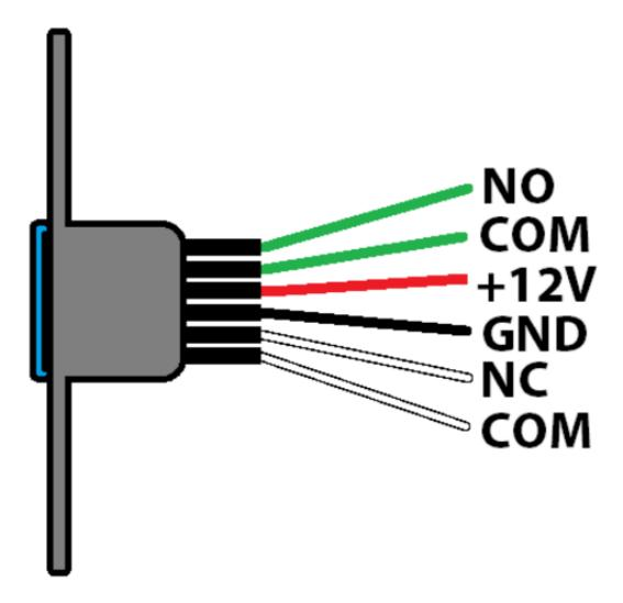
The ACC063 also has a built in blue LED which requires 12V DC (not supplied with the product).
