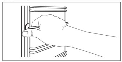
Step 3 Pull the rear end of the shelf support away from the side wall and remove it.
