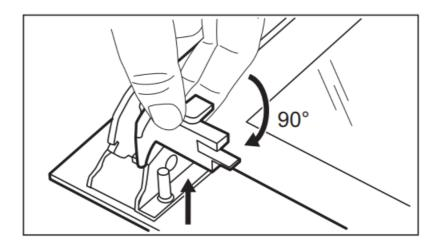
Step 6 First lift carefully and then remove the glass panel.
