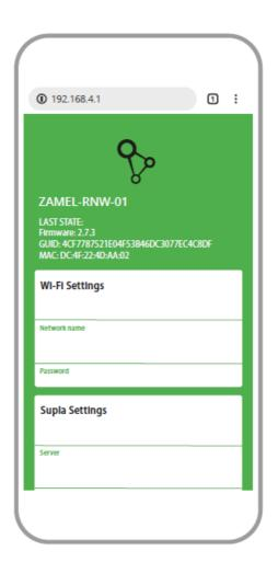
When done, tap "SAVE" at the bottom of the screen. The message "Data saved!" should be displayed. To confirm the entered data, briefly press the CONFIG button on the device. If the device connects to the server successfully, the STATUS LED will go on steadily.
