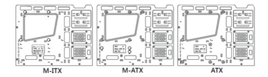
There are 6 Stand-offs preinstalled. Please refer to the diagrams below for additional Stand-Off positions (based on motherboard type).
