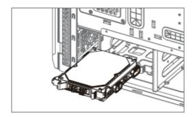
• When transporting an assembled system, Please secure the HDD white Bolt as shown above
