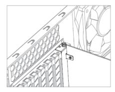
Unfasten the Hand Screw holding the PCI Cover and disassemble the cover. Remove the PCI Slot Cover. Install the VGA Card and fasten it with a fixing screw.
