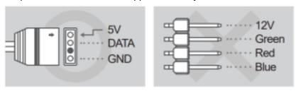
**Caution:** if Addressable 3 Pin connects to 12V header instead of 5V header improperly, It may cause fatal damages to the product by the overvoltage.
