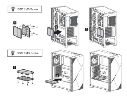
Mounting the 3.5" and 2.5" SSD / HDD
