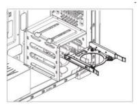
then remove the HDD Tray as shown in the figure.
