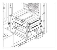
• When transporting an assembled system, please secure the HDD with Bolt as shown above.
