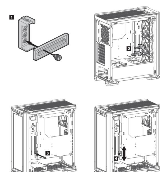
Mounting the 3.5" and 2.5" SSD / HDD
