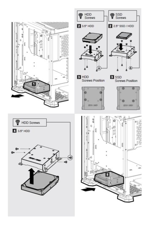
Mounting the 2.5" SSD / HDD
