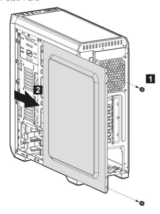
Removing the front panel
