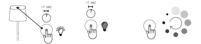
When the lamp is switched on, lightly press the touch sensor to obtain the desired brightness. Every time you turn it on, the light intensity will correspond to the previously set intensity.
