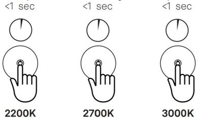
Light pressure for 4 seconds to set the new color temperature and switch off the lamp
