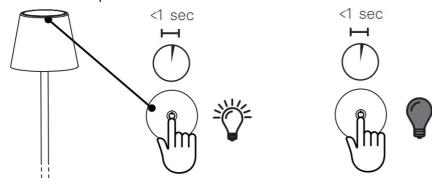
When the lamp is switched on, lightly press the touch sensor to obtain the desired brightness. Every time you turn it on, the light intensity returns to 100%
