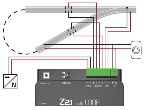
**Tip:** Alternatively the use of track contacts instead of sensor tracks is possible.
