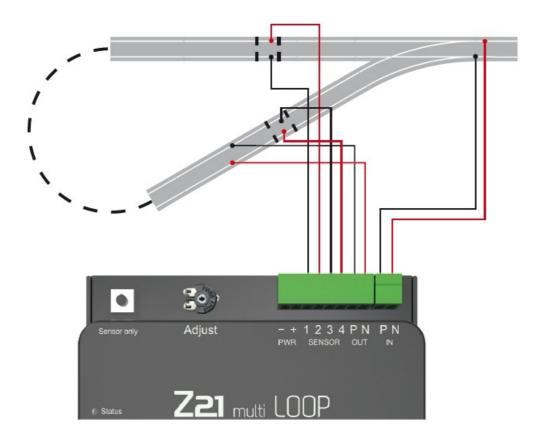
**Tip:** track contacts can be used instead of the sensor tracks. This could possibly improve the interference resistance but necessitates the mounting of a magnet under each of the locomotives so that it can be triggered or you can also use fully configured circuit tracks.
