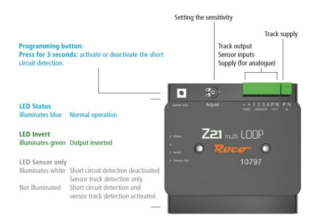
Reversing loops and wye junctions inescapably produce a short circuit at the entry or exit points. There-fore these arrangements require to be electrically isolated at the entry and exit points. To facilitate a reversing loop operation a module is required to take care of the polarization of the loop section.
