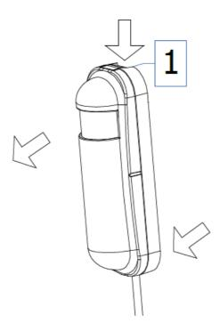
Replace the new battery and install the cover back.
