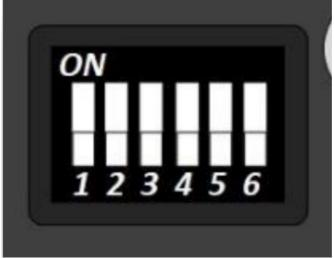
Located on the back side of the unit is a bank of (6) dip switches – you will need a pick-tool to adjust. All dip switches are LIVE, do not unplug the module to adjust.
