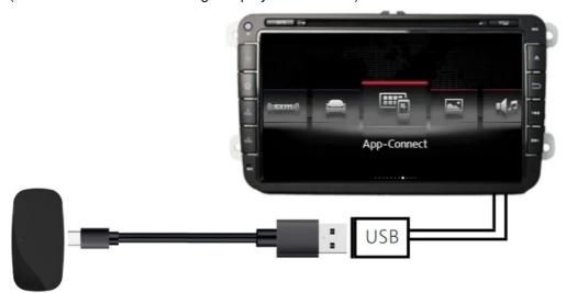
2. Turn on the Bluetooth of the S9-S22, search for the Bluetooth Device naming: "smart Box-\*\*\*\*". Pair it and wait for AA 'Connected to your car'
