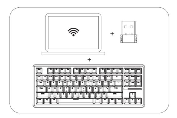
Switch the mode button to 2.4G Mode. Then long press FN+R=2.4G, and the R-key blinks blue. Plug the 2.4G dongle into the computer USB port, then it will pair and install the compatible program automatically. The R-key will stay on and restore to the last RGB mode when paired successfully.
