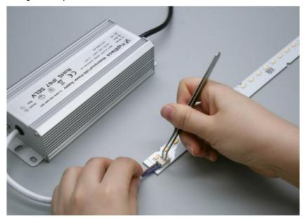
5. Release the push buttons and gently pull the wires to ensure they are securely placed.
