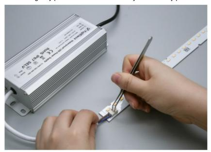
6. For linear daisy-chaining, 10pcs Wago 2060-902 2-pole board-to-board connectors are included in the package. Inset the connectors via push-in terminal blocks for quick and effective linear connectivity.
