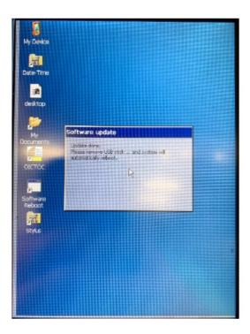
Once completed, simply remove the USB stick and the 1030 Unit will automatically reboot
