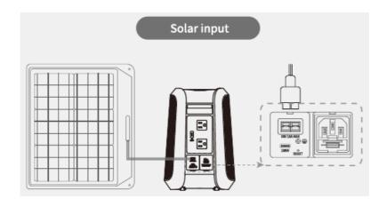
The solar input of 200W max is under optimal sunlight conditions.
