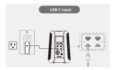
The USB-C Ports (Front panel) are bidirectional output ports, supporting a maximum output/input of 100W.
