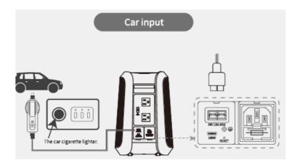
The car charger uses an Anderson interface to the car charger cable.
