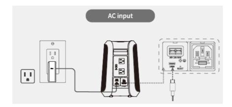
The solar input is 200W max, and the AC Adapter input is 100W max. When both ports are used simultaneously, the total input is limited to 200W.
